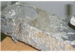
Wave pot assembly erosion
