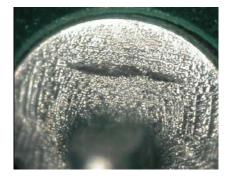
The photo on the left shows the heat tearing effect of tin-silvercopper solder after the wave operation. This tearing effect will not occur on all joints but does occur with all tin-rich solders. It is caused by the rapid cooling of the solder phases incorporating the solder joint. It is not seen in 63/37 joints.
